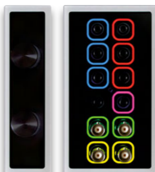
Fig. 4: Intelligent ring socket lighting
