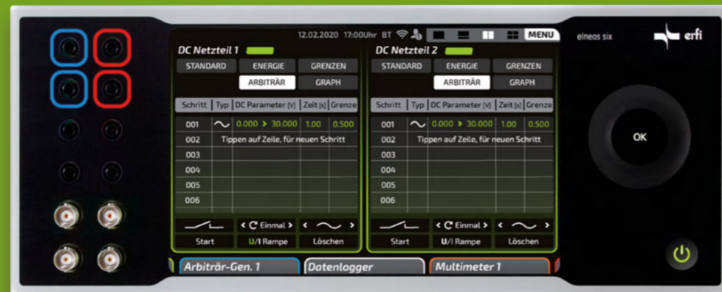
Independent programming: Thanks to variable screen layout, double power arbitrary generators can be programmed independently of each other.
