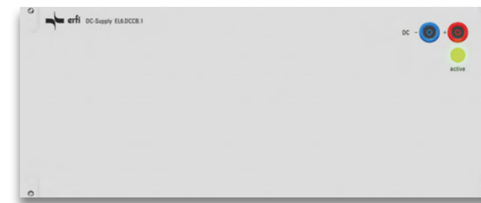
Insert plates with aluminium front for linear DC sources and DC power arbitrary generators 3 U / 63 HP For accommodating a complete DC linear power amplifier incl. power cassette with its own power supply for each device as well as its own backplane for accommodating the DC source. Control by control centre via rear e-bus. Order no. EL6.DCCB.1
