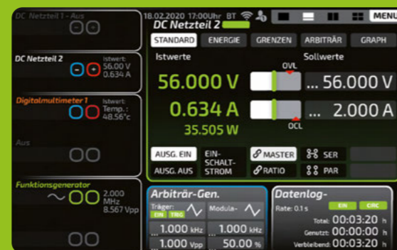
Connection panel and screen scaling: When the connection panels are displayed, all screens move to the right and adapt to the size. The values in the connection panel of the current assignment are clearly visible.
