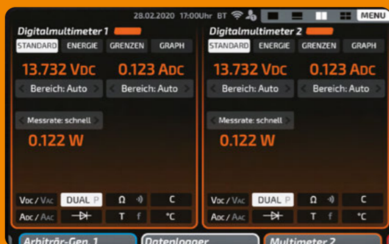
Two digital multimeters in the half-screen: All controls of both digital multimeters can be operated simultaneously and independently of each other. The optional dual measurement allows each digital multimeter to measure current and voltage in the AC and DC range simultaneously.
