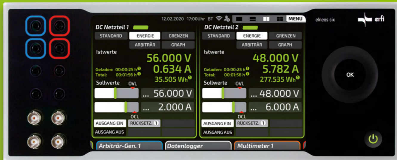
Halfscreen: A dual power supply unit can be operated by several users at the same time through the split screen. The device selection bar at the edge of the screen allows access to other devices.
