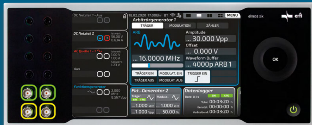
New connection panel: The panel slides into the screen by a swipe gesture from the right and the other screen contents contract. In this way, all connections remain visible and operable when the connection panel is displayed.
