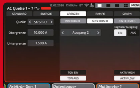
Limiter: The limiter allows free monitoring of voltage and current ranges in connection with limits. Each state can be coupled with an acoustic signal and a freely selectable digital output.
