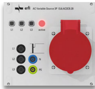
Alufront AC source 3-phase not ungrounded, 3 U / 28 HP Output (secured): 5 SLS 1 , 1 CEE socket 16 A Display: RGB-LED for Output active Order no. EL6.AC3CB.20
