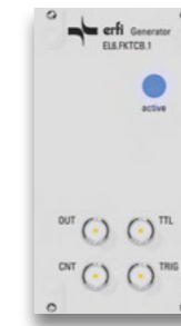
Slave as aluminium front for function generator and fast signal arbitrary generator 3 U / 14 HP To accommodate 1 function generator EL6.F or 1 fast signal arbitrary generator incl. EL6.S function generator. Control by control centre via rear e-bus. Input: 2 BNC sockets for counter and trigger Output: 2 BNC sockets for OUT and TTL Display: RGB-LED for device active Order no. EL6.FKTCB.1
