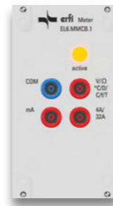
Slave as aluminium front for digital multimeter and power meter 3 U / 14 HP To accommodate 1 digital multimeter EL6.D or 1 power meter incl. digital multimeter EL6.P. Control by control centre via rear e-bus. Input: 4 SLS 1 for all measurands Display: RGB-LED for device active Order no. EL6.MMCB.1
