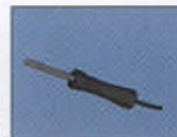
Protective conductor probe
