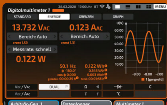
More scalable graphic measured value display: In the upper half, the power meter displays all measurement data. At the same time, in full-screen mode, other devices can be displayed in the smart scroll bar.
