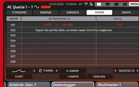
Ramp generator: The 8-inch display allows any sequences to be entered directly without any programming effort. Alternatively, the sequences can be transferred and started via the interface.
