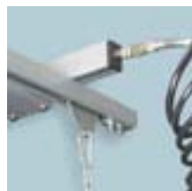
The direct connection of the air-operated tools: Air-operated tools can be connected directly with the compressed air coupling which is installed in the extension arm.
